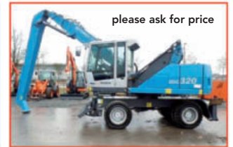
Fuchs MHL320 D 2013, 10.4 m reach, 19 t, stabilizer blade, high lift cabin and 2-p-stabilizer
