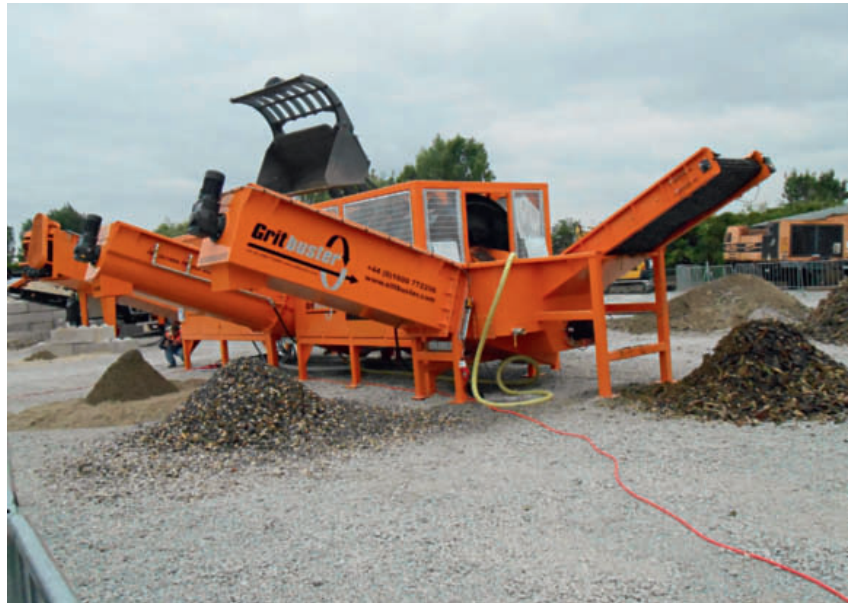
▲ Gritbuster – Washing drum with sand auger and stone auger
