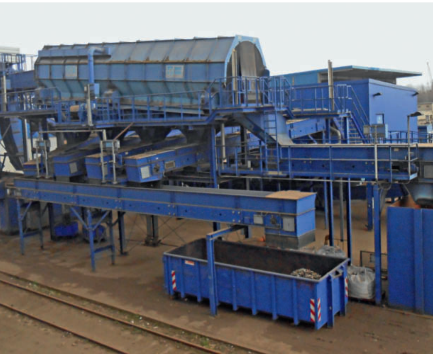
From the mega shredder ▲ non-ferrous fractions go to the sorting lines for further treatment
