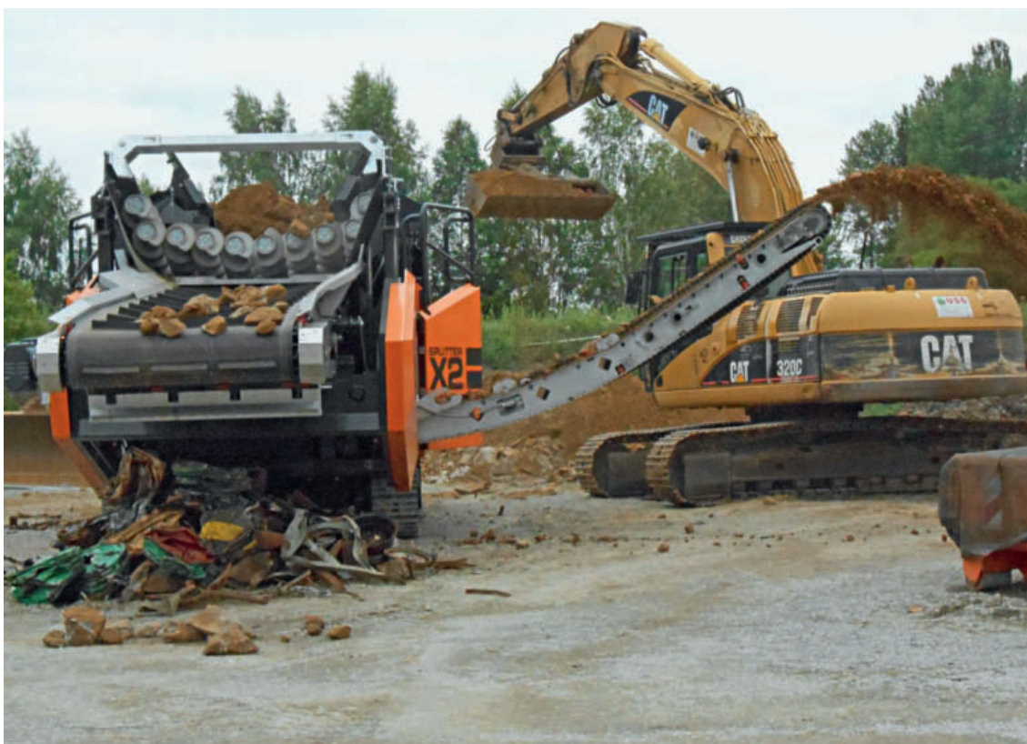
◀ Splitter X2 – mobile spiral shaft separator on tracklaying chassis
