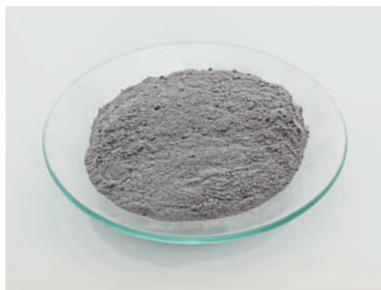
7 Separation of the semiconductor film from the front glass and concentration in the fines fraction
