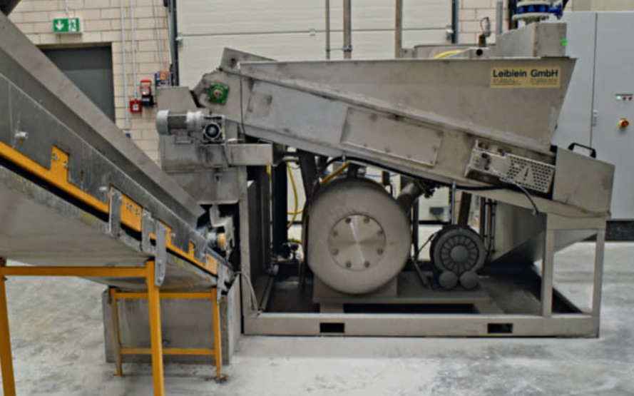
Side view of the vacuum band filter from Leiblein
