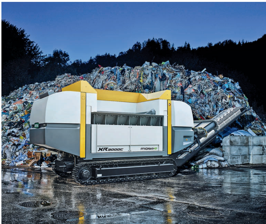
◀ Electrically-driven mobile shredder XR mobil-e with a low power electric drive
