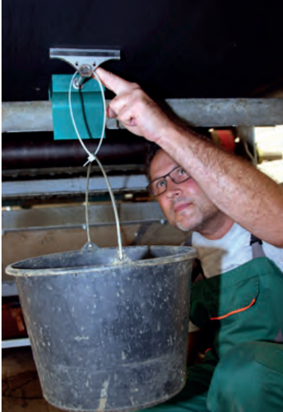
◀ Andreas Griesser, service employee of Schulte Strathaus, during the demonstration of the measuring process „Scraper Performance Test“ for the competition
