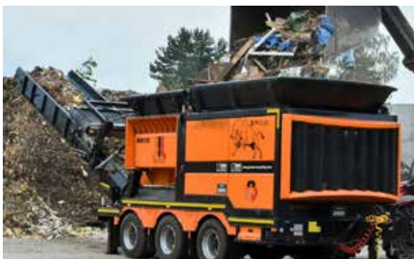
▲ MRW 2.85 twin-shaft shredder: flexible, fast, mounted on wheels for easy transport MRW 2.85 Doppelwellenzerkleinerer: flexibel, schnell, schonend auf Rad
